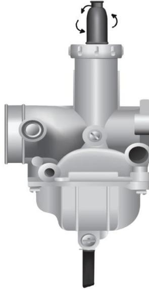
**Step 4:** In some cases it may be necessary to remove material from the cast stop in the carburetor cap. Material can easily be removed with simple sand paper around a flat bar, or a small file after only a few passes. Make sure to remove the gasket prior to sanding, placing it back onto the cap during reassembly.
