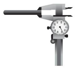
• Each slide is identified by color along with a reference to maximum allowable opening. This maximum opening is measured from the base (floor) of the carburetor bore to the <u>front</u> lip of the throttle slide.
