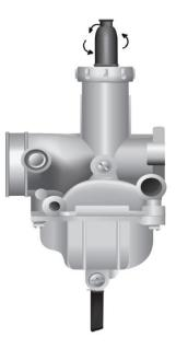
**Step 4:** In some cases it may be necessary to remove material from the cast stop in the carburetor cap. Material can easily be removed with simple sand paper around a flat bar, or a small file after only a few passes. Make sure to remove the gasket prior to sanding, placing it back onto the cap during reassembly.
