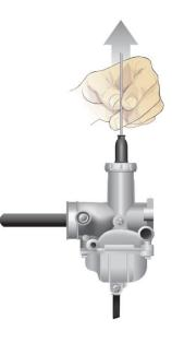
**Step 6**: Install locking cap, tighten, and recheck.
